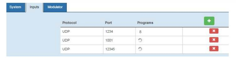
In the first step, the IP address, netmask and gateway address of stream sources are assigned to the ETHERNET interface for use in the local network. And Port number of streams are individualized!
