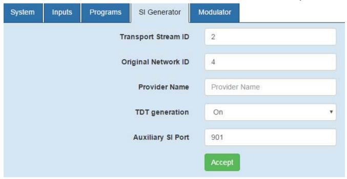
Every service in a DVB network can be uniquely identified by three values. These values are the Original Network ID (the ID of the network that originally broadcast the service), the Transport Stream ID (to identify a particular transport stream from that network) and a Service ID to identify a service within that transport stream.
