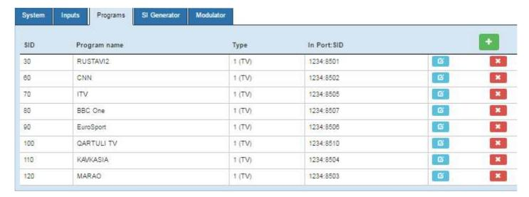
The position information that was specified in the configuration will form the basis for the allocation of PID Service IDs in ascending order. You can change program names, A PID, VPID, SID and TYPE OF PROGRAM (1-TV, 2-Radio, 3-Teletext, 4-Unknown). VPID and PCR-PID has a same value.
