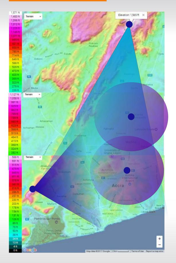
Terrestrial microwave broadcasting implies the obligatory presence of the line of sight between transmitting antenna and receiving antenna of MVDS system subscriber. Fitting locations of repeaters and signal coverage area indicated in the Figure 1.
