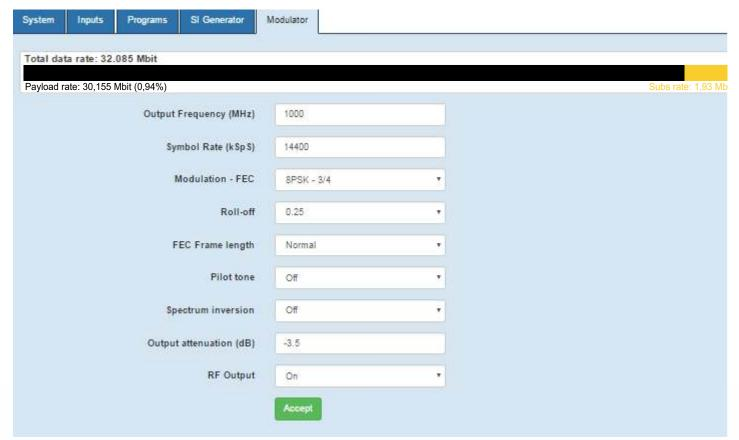
The actual bitrate at the output of the modulator is displayed as a blue scale at the top of the menu. Free capacity of the transponder is filled with zero packets if the subscription data does not come to the modulator from the billing server. The capacity occupied by zero packets is indicated in the form of a gray scale.
